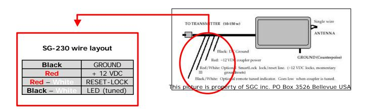
The **RED** and the **BLACK** wires connect to the 12 VDC power supply.
