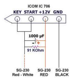
The reason for bridging pin 1 to pin 2 on the IC-706 is that we want to fool the IC-706 thinking that there is a remote tuner (Icom model) present. By wiring pin 1 to pin 2 the START pin (2) is pulled high.
