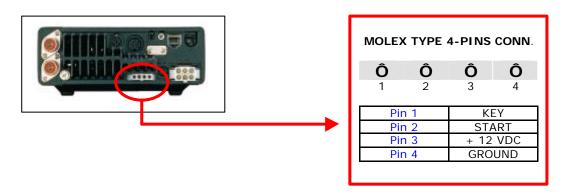
**Pin 3** and **pin 4** provide DC output to power the SG-230. By using the DC power supply in this connector the SG-230 automatically powers on and off when switching the IC-706 on or off.
